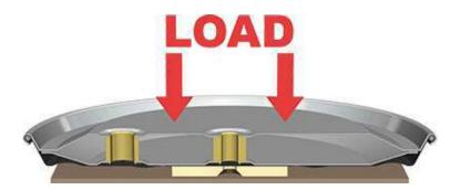
A controlled 'leakage' of the compressed air creates a thin air film between the floor and the air caster.
