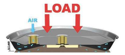
The air caster now floats with an air film, so there is practically no friction and it is possible to easily move heavy objects with little force.
