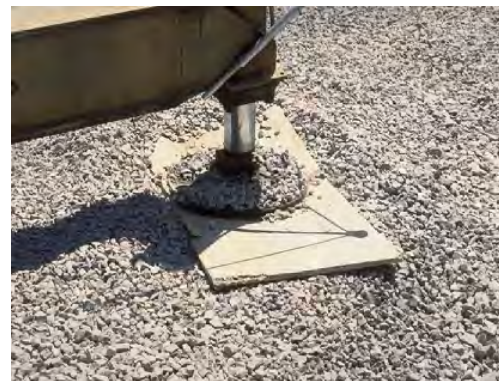
Figure D2 - Examples of Outrigger Pads with Insufficient Stiffness
