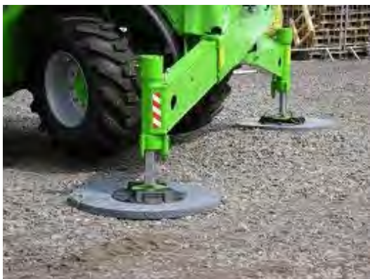
Telehandler Outriggers on Round Pads
