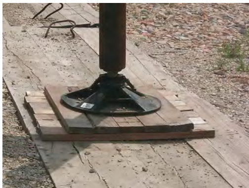
Figure D2 - Examples of Outrigger Pads with Insufficient Stiffness
